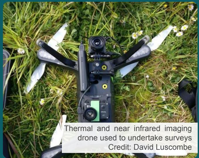
Thermal and near infrared imaging drone used to undertake surveys
